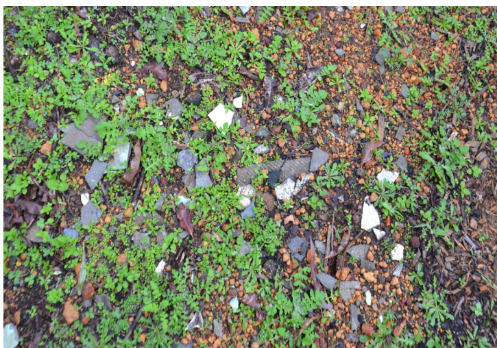
Figure 11 Hot spot of bonded asbestos cement fragments.
